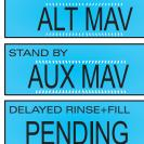
"DELAYED RINSE+FILL" is displayed whenever a zero-capacity tank has transferred to an off-line state and is currently waiting to initiate the second portion of a regeneration cycle. Viewed only when Delayed Rinse and Fill is set to ON.
